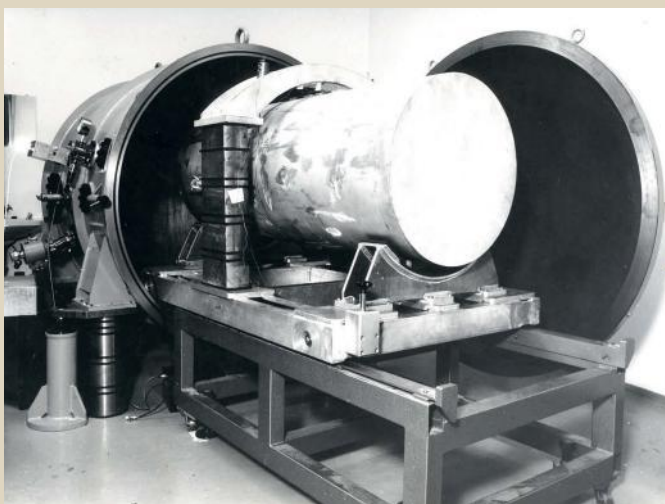
Weighty experiment: In the early 1970s, Max Planck researchers used a massive aluminum cylinder like the one shown here in their search for gravitational waves.
