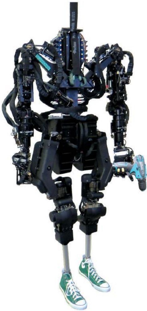
A Goddess in Chucks: Athena uses hydraulics to move her limbs when handling a tool or walking. She may not have a head, but she's wearing trendy sneakers.
